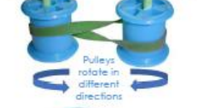
Pulleys rotate in different directions
